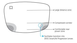
Single vision wearers near point Based on reading behavior, the near point location is located higher than for progressive lens wearers.
